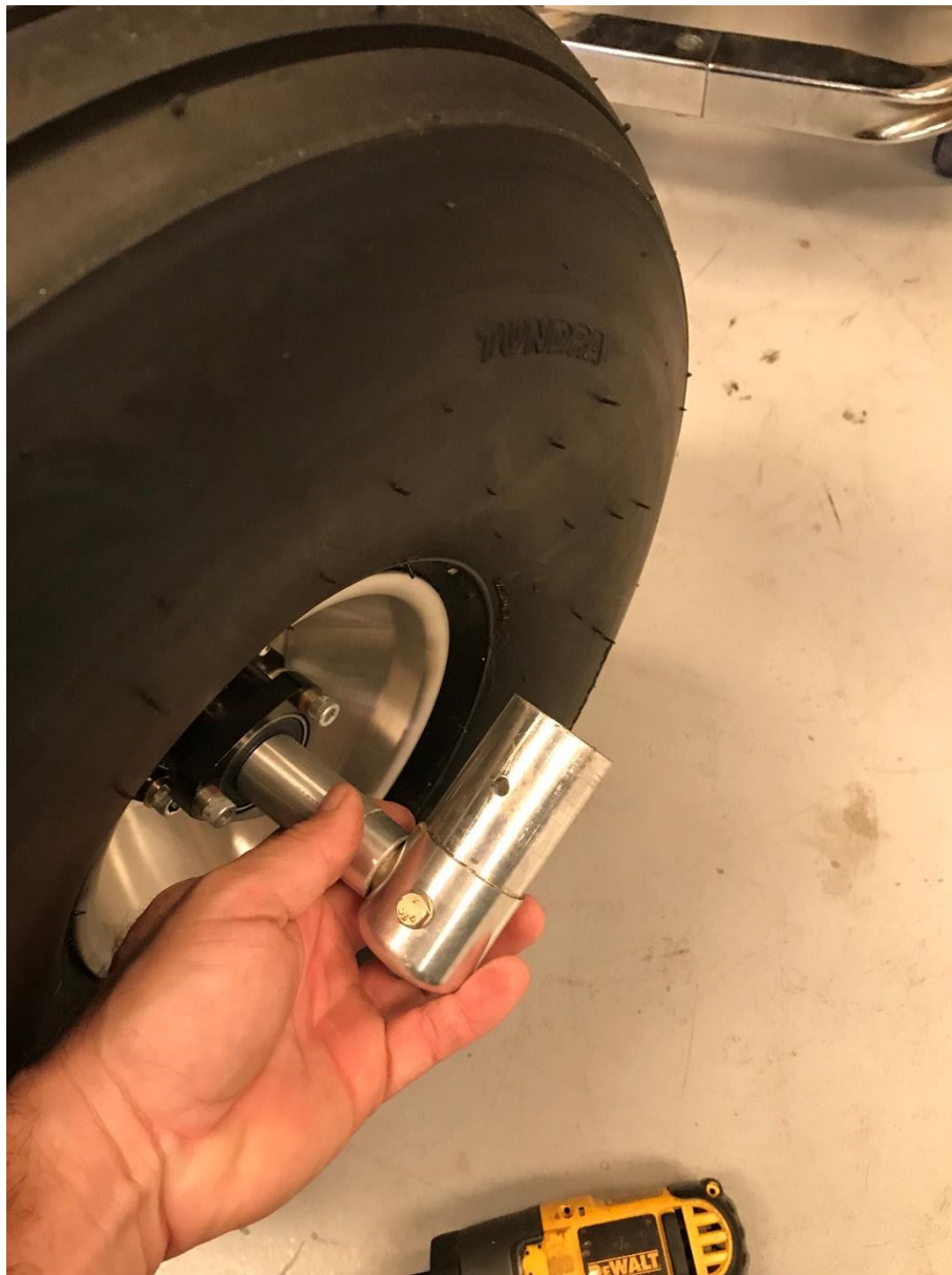
Through Bolt Secures Axle
