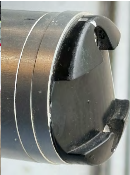
Tip Cap pressed down into the Shim and alum edge can cut the Webbing
