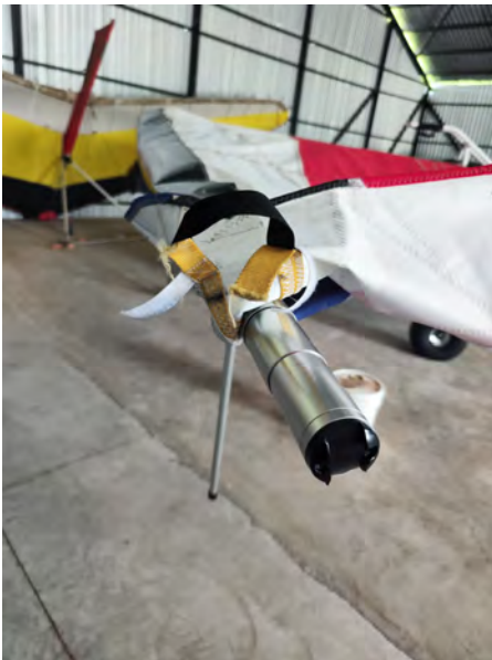
Tip Cap pressed down into the Shim and alum edge can cut the Webbing
