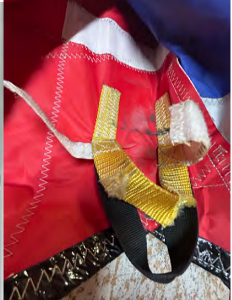
Tip Cap pressed down into the Shim and alum edge can cut the Webbing
