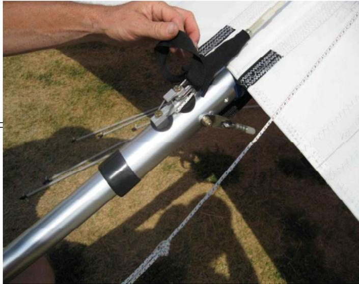
**8. INSERT REMAINING BATTENS** Remove the tip bags and insert remaining 3 top surface battens towards the wing tips, then lastly the straight spring loaded tip battens onto LE hooks. Cordless battens hook in a bit differently than traditional corded battens. See pictures below.
