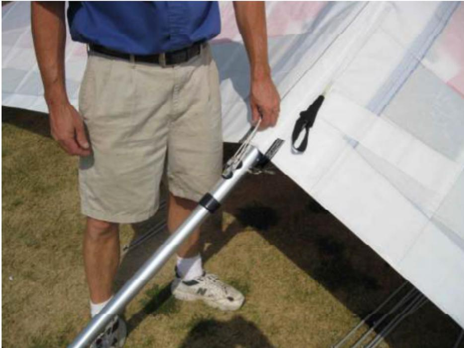
6. INSTALL STRUTS Place struts under wing on each side. There is a left and right strut and are marked. The strut also should be marked top. This is the side that has a 5/16" clevis pin. First hook up the lower end of the strut (bolt, castle nut and safety pin) then the top. Make sure you install the safety rings and make sure that the safety rings.
