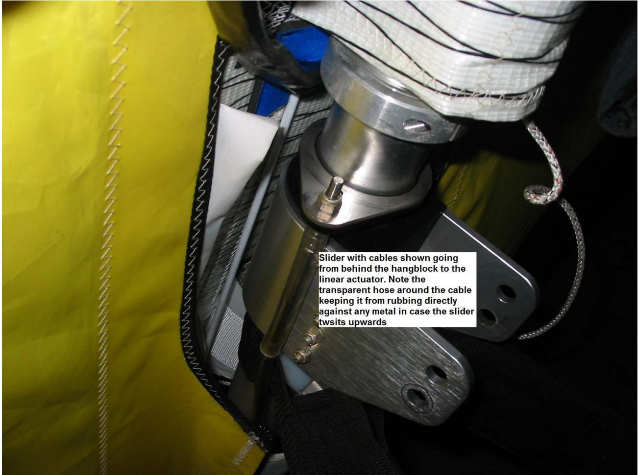
Slider with cables shown going from behind the hangblock to the linear actuator. Note the transparent hose around the cable keeping it from rubbing directly against any metal in case the slider twsits upwards
