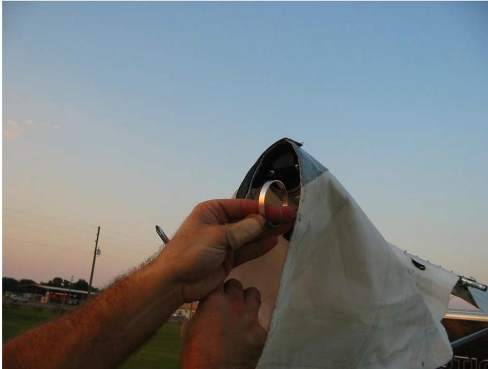
Make sure the screws are in-line with the mark on the LE when it was removed. The rotation of these caps is very important!
