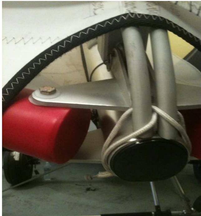
13. POSITION THE NOSE BATTEN AND NOSE CONE Pull the nose down to eye level so you can put the nose rib on the 1/4" stud located front top of keel tube. With nose cone in hand start with the two top Velcro tabs and gently pull the nose cone down and around the nose plate to connect the two bottom Velcro tabs on the nose cone to its corresponding Velcro sewn on the under surface below the keel.
