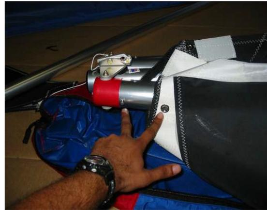
Note: After the wing is completely set up and you have put in the center battens you can reinstall the sail nose screws.
