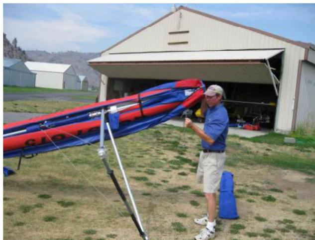
**3. ATTACH THE FRONT FLYING WIRES** Ensure that all the lower rigging is untangled first.
