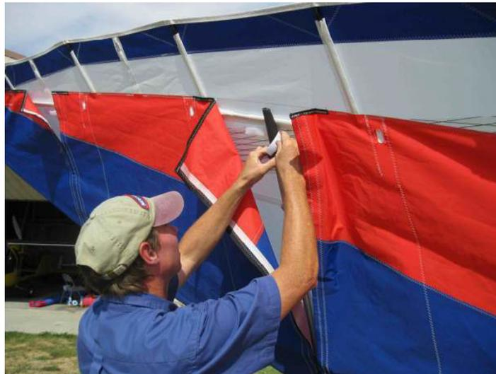
10. UNDER SURFACE BATTENS Install the under surface battens from longest to shortest. Make sure the back ends are inserted back into the slot at the rear.
