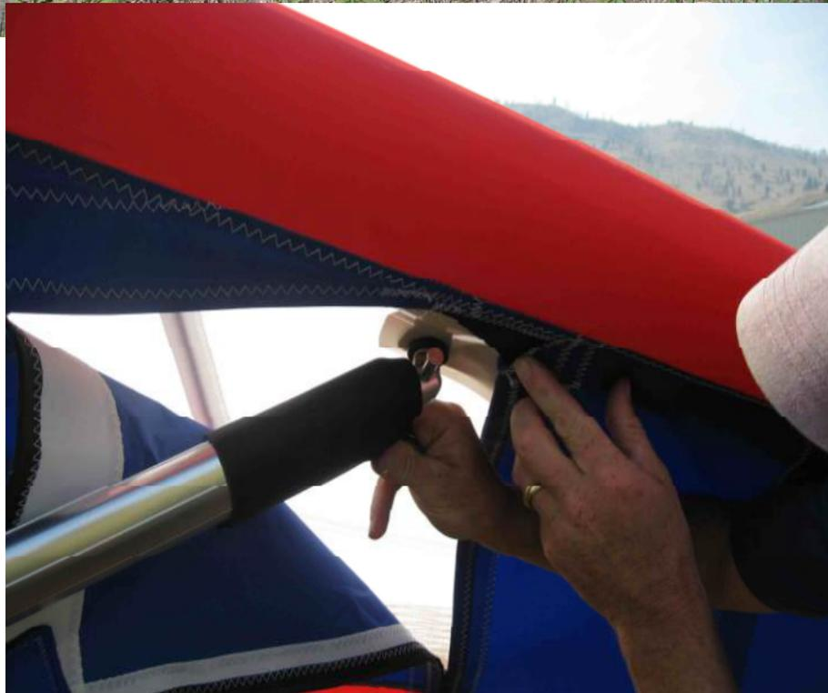
**7. HOOK UP THE CROSS BAR MAIN CABLE** Remove pull back nylon line from spring catch. Pull the line all the way back, until you can latch the cable shackle into the spring catch. Make sure the wing tip yellow webbing is completely in the 1" slot on the wing tip cap before tightening the wing with the haul-back cable.
