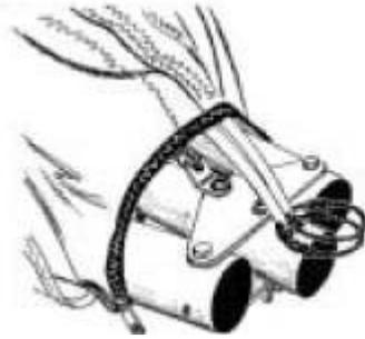
After closing the wing, the frame can now be snaked out through the nose of the sail.
