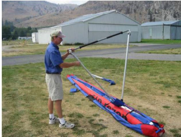
2. ROLL THE WING OVER Stand wing on the control frame (do not attach the lower front control frame wires at this time). Note the assembled A Frame will try to fall over and turn 90 degrees to its proper orientation. Try to limit the amount of stress put on the upper down tube connection FIG.3
