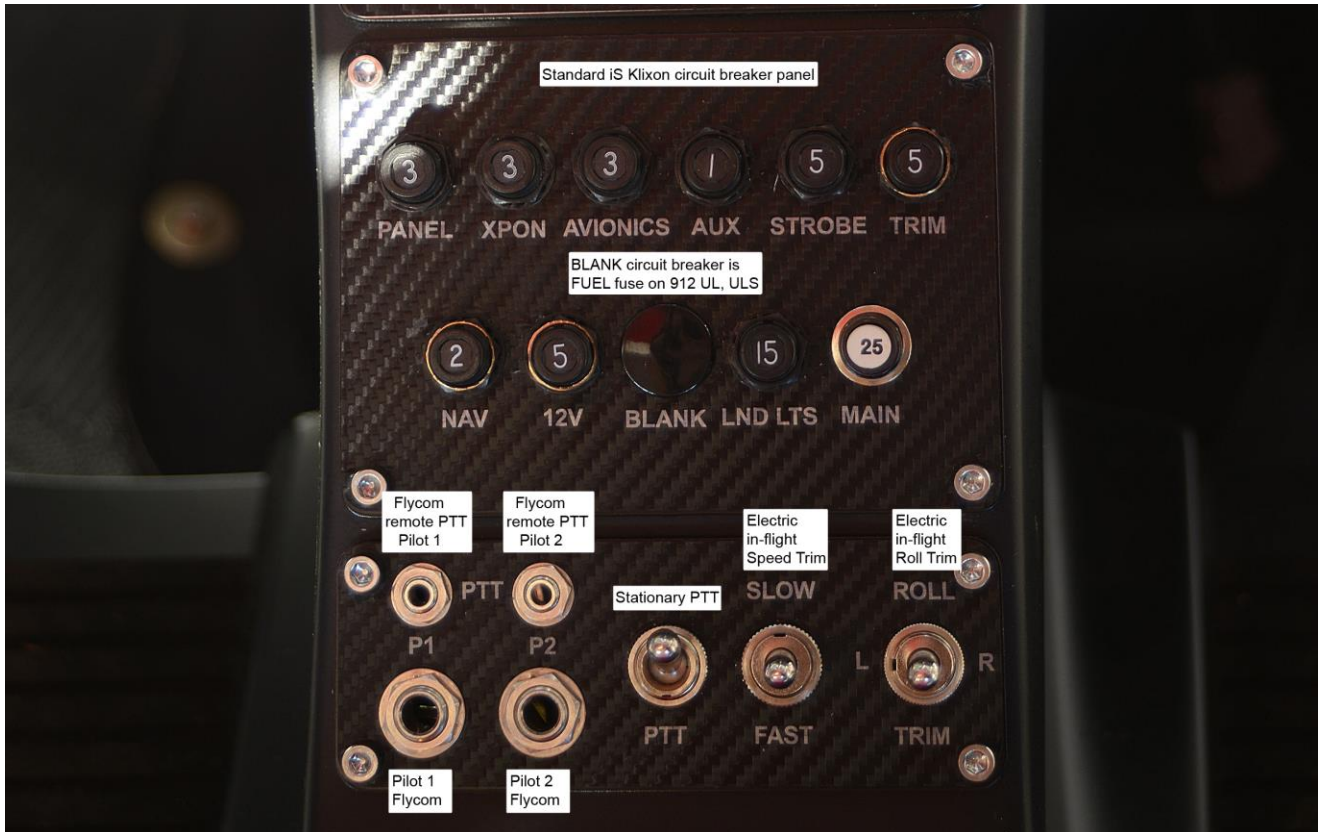
Standard Circuit Breaker/ PTT Panel for 912 UL, ULS, iS with the iS switch panel
