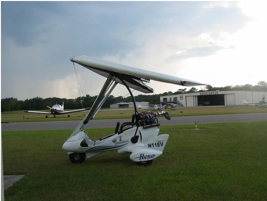
The Revo trike carriage is a two seat tandem WSC aircraft. The layout is typical for two seat trike design, with the pilot, passenger and pod being suspended by a triangular frame made of 4130 aircraft Chrome moly MIG welded and de-stressed to aircraft standards, hanging from the top of the 4130 Chrome moly mast about the pitch and roll axes, to provide for weight shift control.
