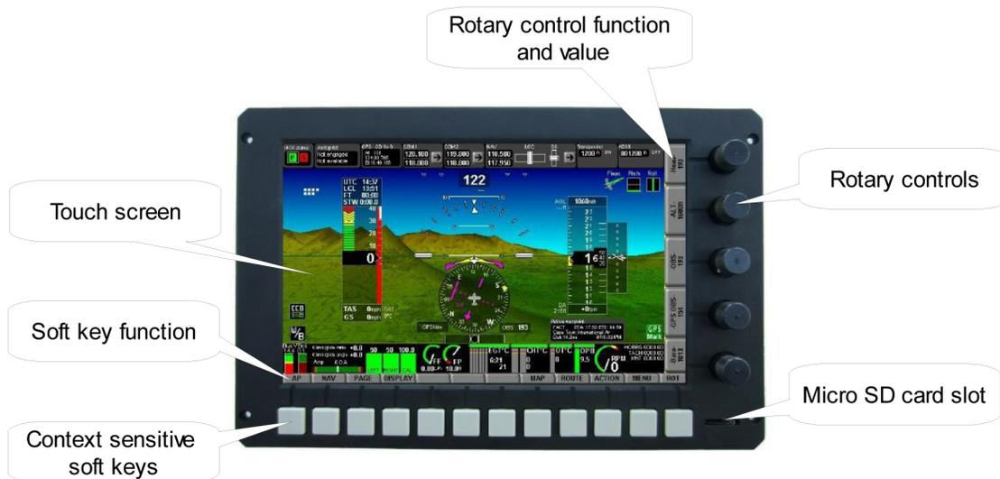
The 8.5" Explorer iEFIS is an option for all 912 engine configurations. The iEFIS utilizes a custom developed, pressure sensitive, sunlight readable touchscreen that can also be operated using gloves. The iEFIS screens can be completely edited by the user using a simple PC program to create various displays.
