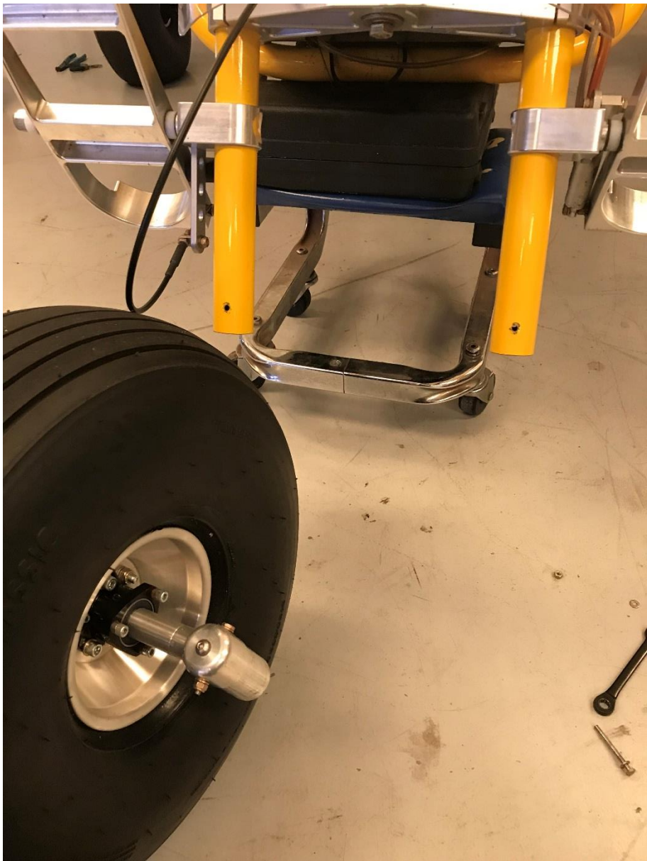
Lower Fork Fittings Removed
