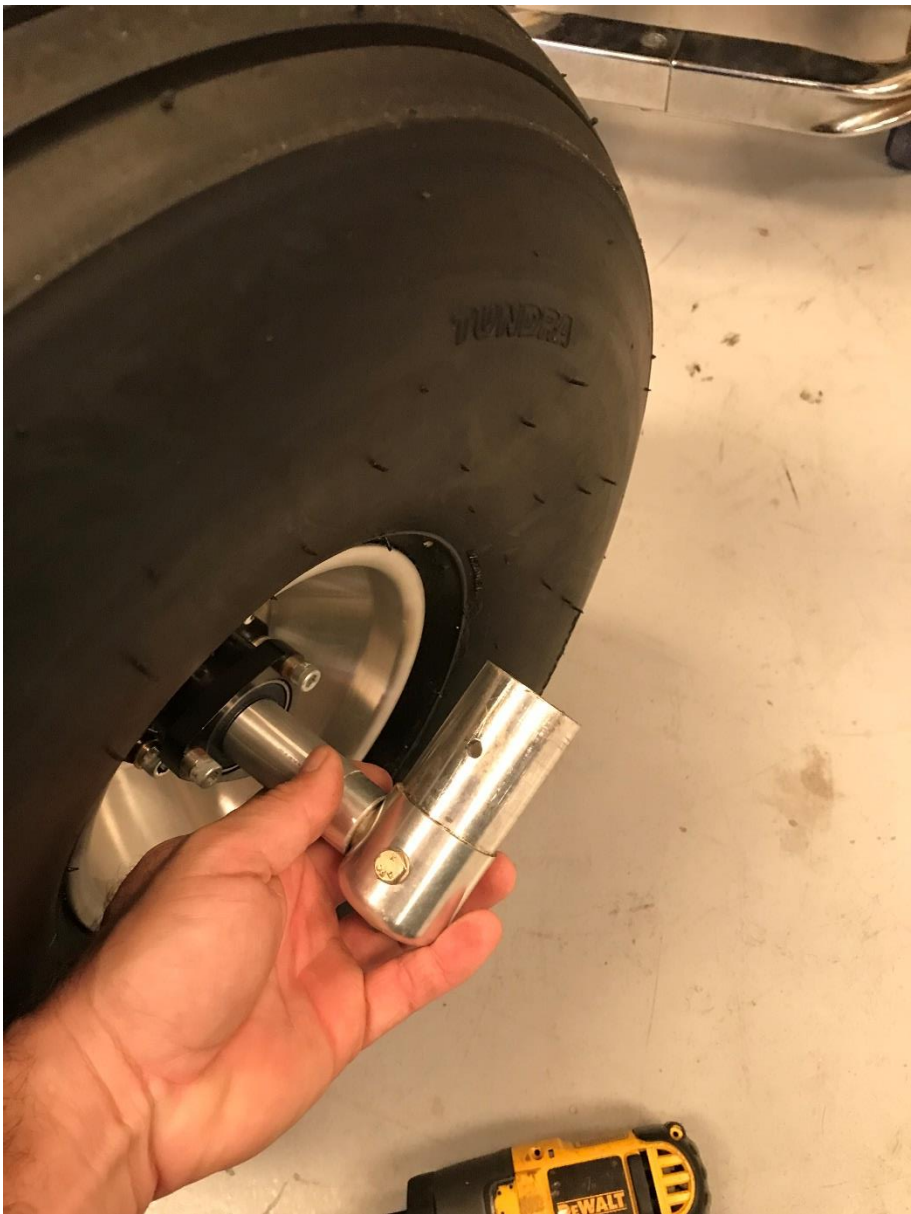
Through Bolt Secures Axle
