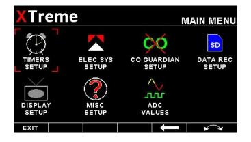
The XTreme EMS is used when the 912 IS is chosen. It is a 4.3" sunlight readable, wide viewing angle, high resolution LCD display. It integrates an SD card reader (for software updates and for engine data recorder), 5 function buttons, a rotary control.
