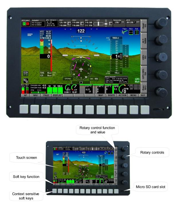
The 8.5" Explorer iEFIS is an option for all 912 engine configurations. The iEFIS utilizes a custom developed, pressure sensitive, sunlight readable touchscreen that can also be operated using gloves. The iEFIS screens can be completely edited by the user using a simple PC program to create various displays.
