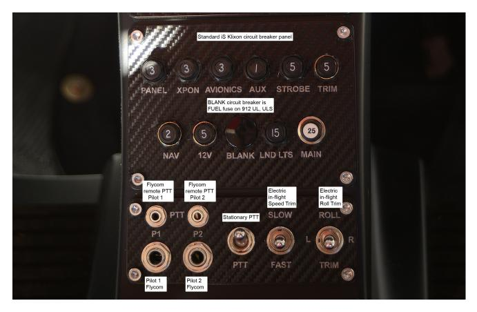
Standard Circuit Breaker/ PTT Panel for 912 UL, ULS, iS with the iS switch panel
