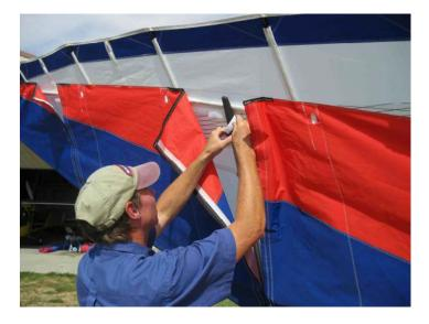
10. <u>UNDER SURFACE BATTENS</u> Install the under surface battens from longest to shortest. Make sure the back ends are inserted back into the slot at the rear.
