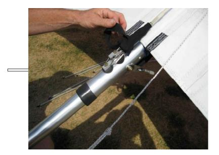
8. <u>INSERT REMAINING BATTENS</u> Remove the tip bags and insert remaining 3 top surface battens towards the wing tips, then lastly the straight spring loaded tip battens onto LE hooks. Cordless battens hook in a bit differently than traditional corded battens. See pictures below.
