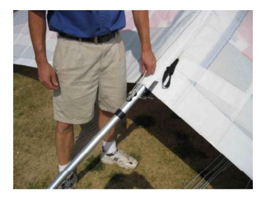
6. <u>INSTALL STRUTS</u> Place struts under wing on each side. There is a left and right strut and are marked. The strut also should be marked top. This is the side that has a 5/16" clevis pin. First hook up the lower end of the strut (bolt, castle nut and safety pin) then the top. Make sure you install the safety rings and make sure that the safety rings.
