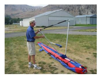
2. <u>ROLL THE WING OVER</u> Stand wing on the control frame (do not attach the lower front control frame wires at this time). Note the assembled A Frame will try to fall over and turn 90 degrees to its proper orientation. Try to limit the amount of stress put on the upper down tube connection FIG.3
