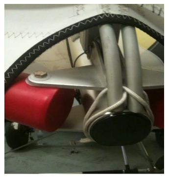
13. <u>POSITION THE NOSE BATTEN AND NOSE CONE</u> Pull the nose down to eye level so you can put the nose rib on the 1/4" stud located front top of keel tube. With nose cone in hand start with the two top Velcro tabs and gently pull the nose cone down and around the nose plate to connect the two bottom Velcro tabs on the nose cone to its corresponding Velcro sewn on the under surface below the keel.
